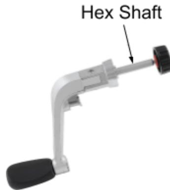
To connect our stepper motor to the spinning reel, we will join a hexagonal shaft to our stepper motor's shaft using a coupling. The hexagonal shaft will slide into the reel's slot where the original hand crank shaft was placed. Finally, the stepper motor will be mounted to the fishing reel. A spinning reel can spin in both directions (reeling in/out), so we can control the depth of our line by reversing the direction of the stepper motor to either raise or lower the lure.
