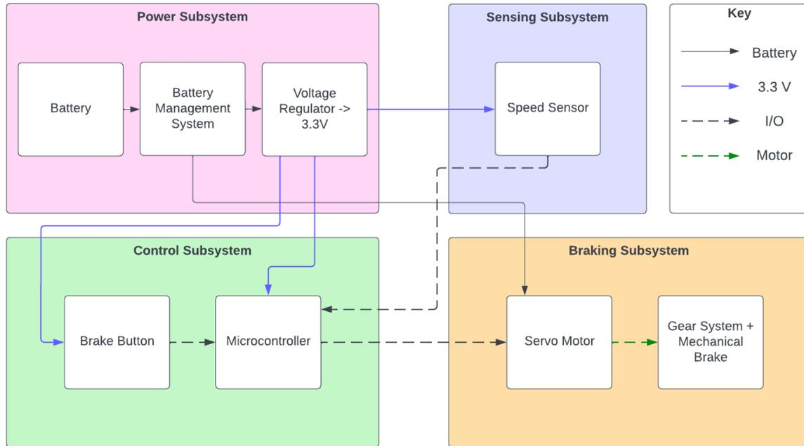
Figure 2: Block diagram of the anti-lock braking system.
