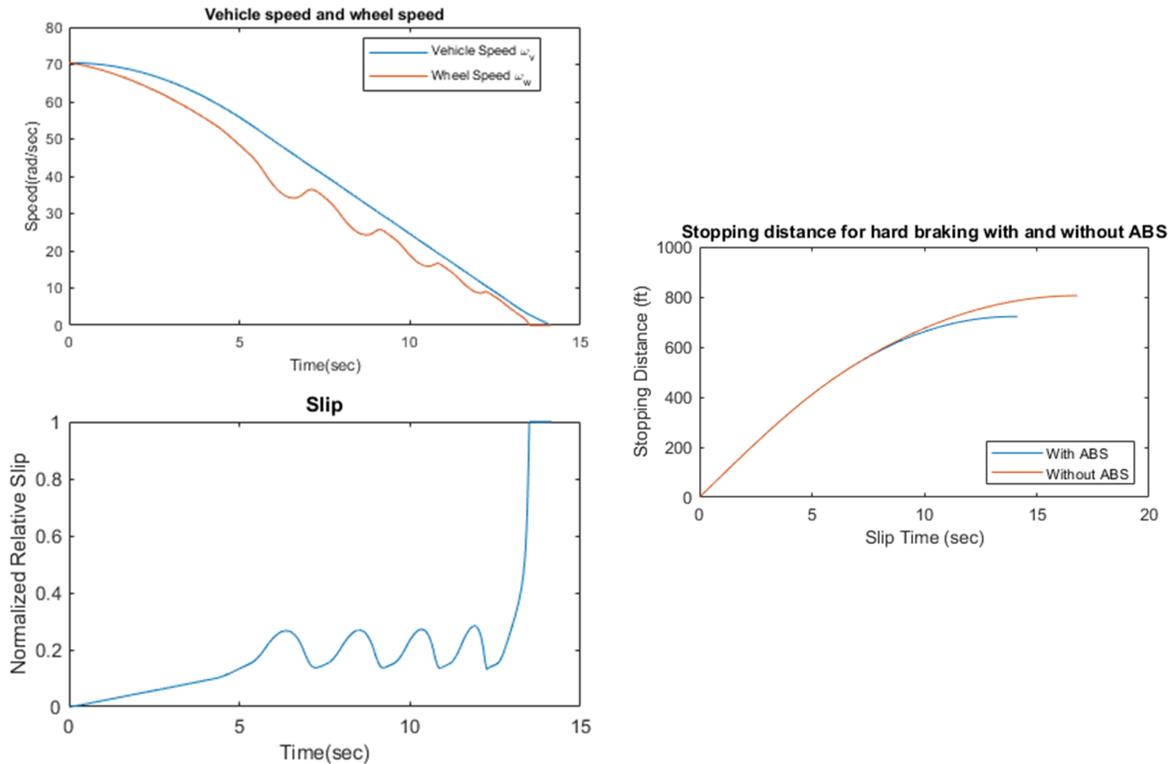
Figure 5: MathWorks Simulation of Car ABS
