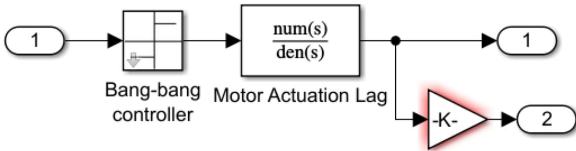
Figure 4: Prototype Motor Controller
