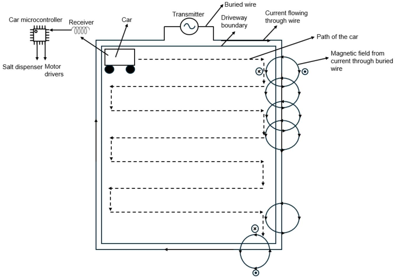
Figure 1: Movement of the car around the driveway and position of wire around the driveway
