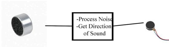
Microcontroller Recovers Direction of sound, Processes the noise and outputs signal to motors
