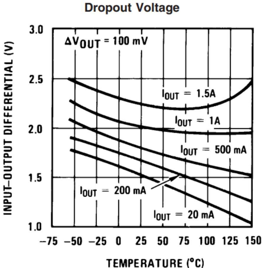
Figure 6. Temperature vs. Dropout Voltage at various load currents
