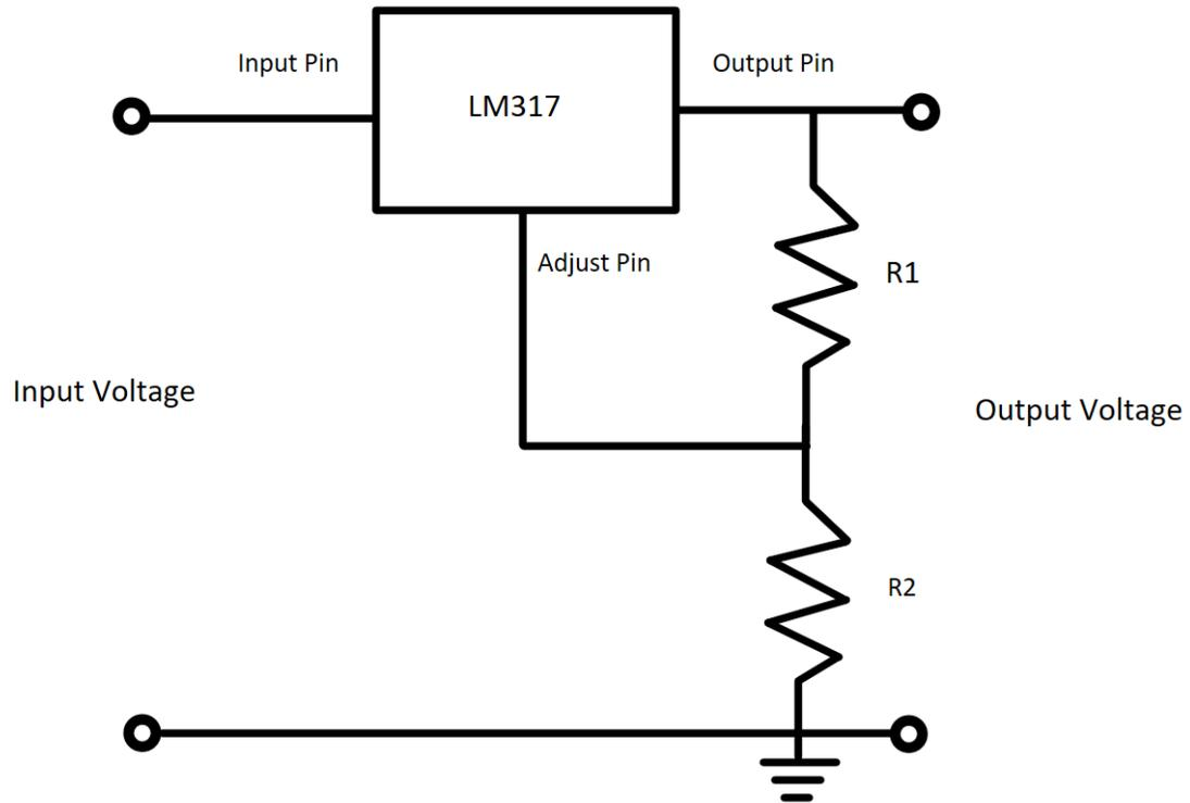
Figure 5. LM317 voltage regulator
