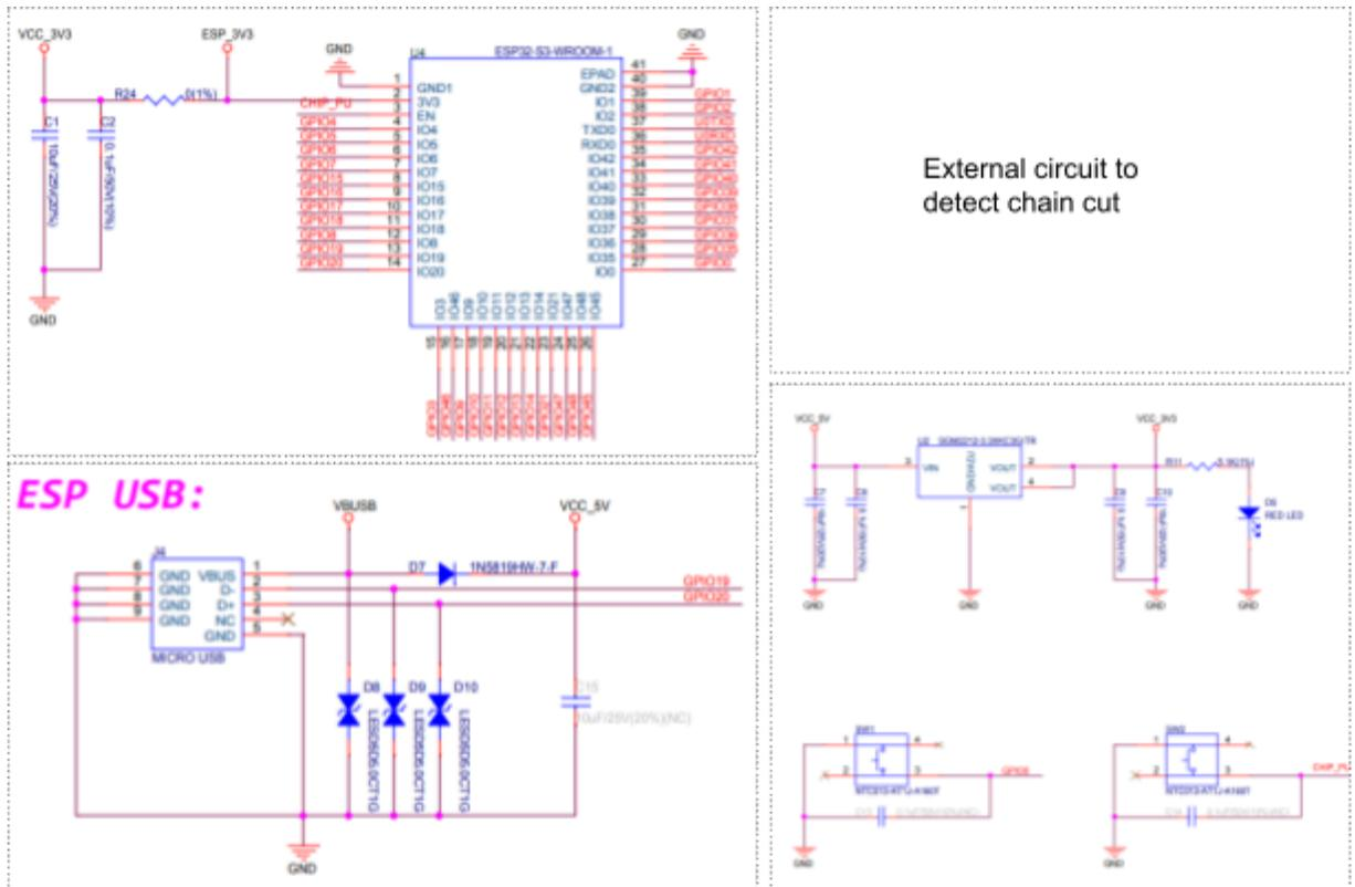
Figure 4. Draft of Schematic (Source: Espressif) [9]
