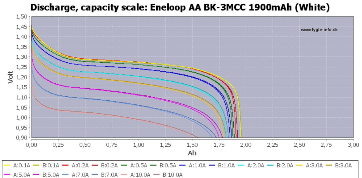
Figure 7. Discharge profile of 1.5V AA BK-3MCC battery
