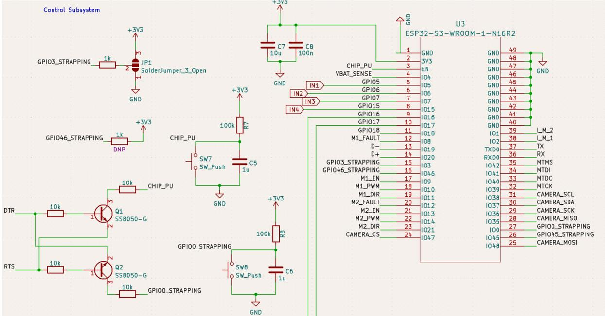
Figure 11: Prototype Control System for ESP32
