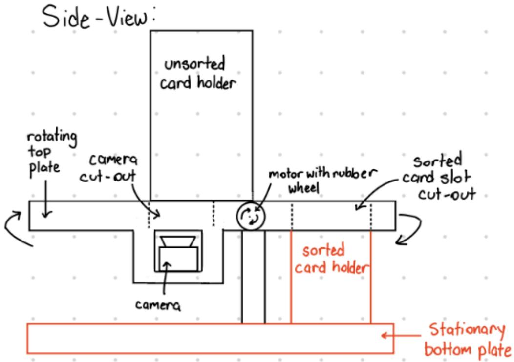
Figure 3: Physical Side view of Design
