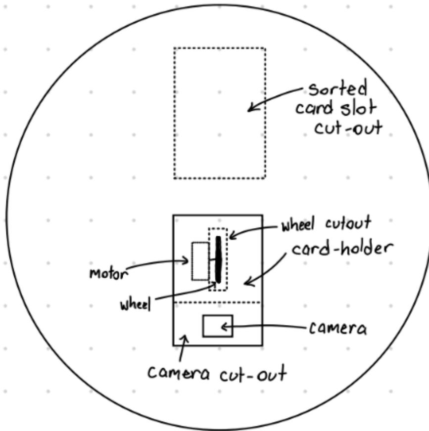
Figure 4: Physical Top view of Top Plate
