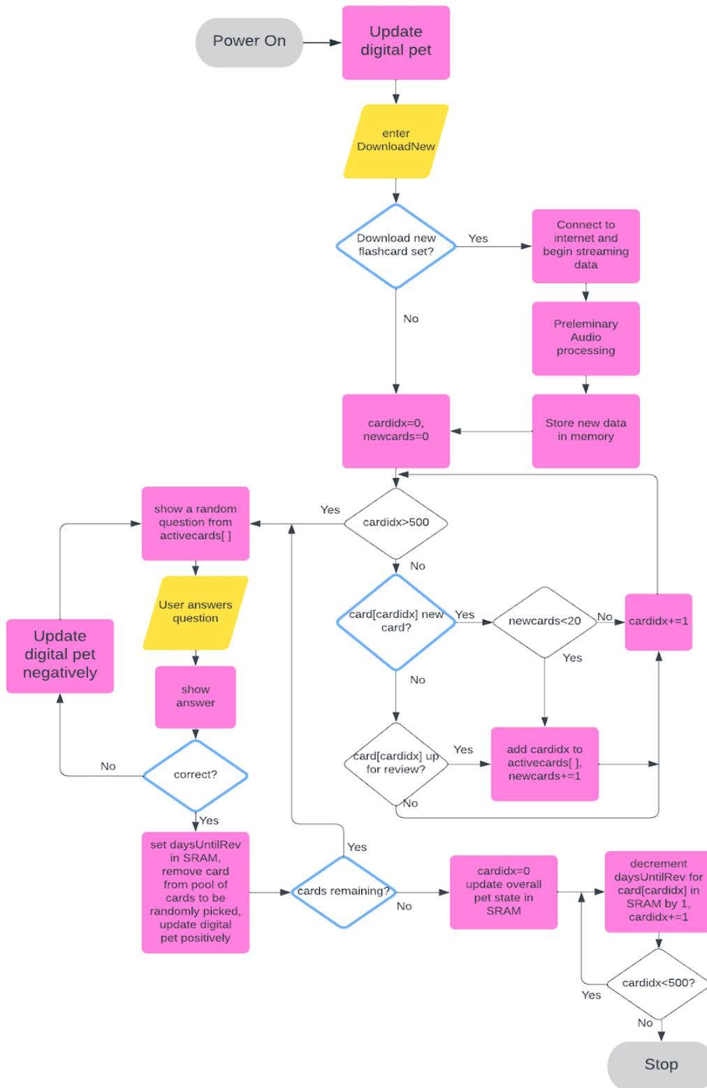
Figure 5: High level MCU algorithm flowchart
