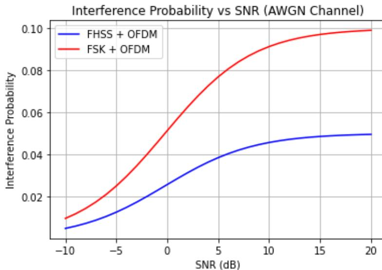
Figure 1: Probability of Frequency Dependent Interference versus SNR
