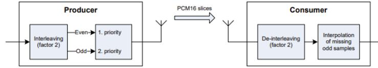
Figure 4: PCM16 Processing Diagram
