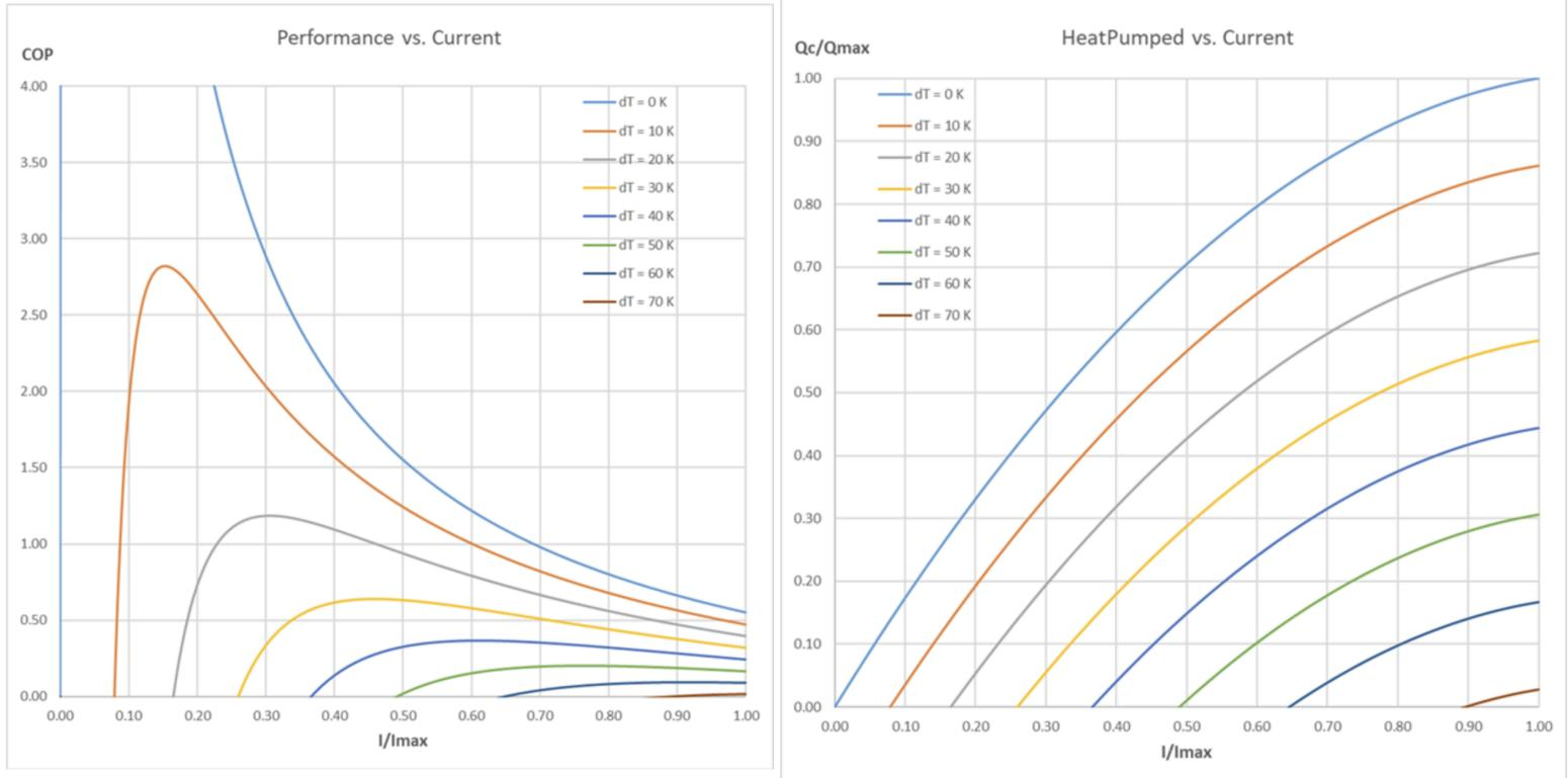
Figures 3 and 4: COP efficiency and Heating Power vs Current trends
