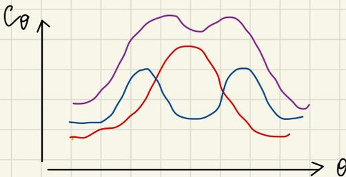
$$GCC-Phat(x, y, f) = \frac{a_i^* X(f) Y(f)}{\|X(f) Y(f)\|} \quad \text{GCC}$$
