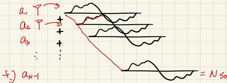
② For max SNR at  $R_x$ , *compensate phase shift  $\phi_i$*
