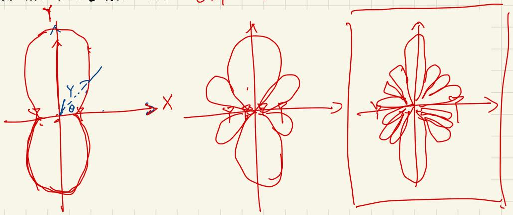
④ Observe, the natural beam is pointing towards Front and Back antennas transmit same signal
