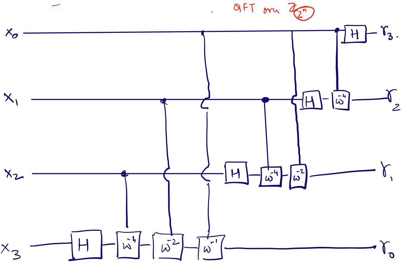
where  $\omega^{-4} = \begin{bmatrix} 1 & 0 \\ 0 & \omega^{-4} \end{bmatrix}$      $\omega^{-2} = \begin{bmatrix} 1 & 0 \\ 0 & \omega^{-2} \end{bmatrix}$
