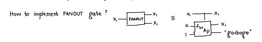
Corollary Any classical circuit computing F: {0,13" → {0,13" can be efficiently converted to a reversible (and hence quantum) circuit
