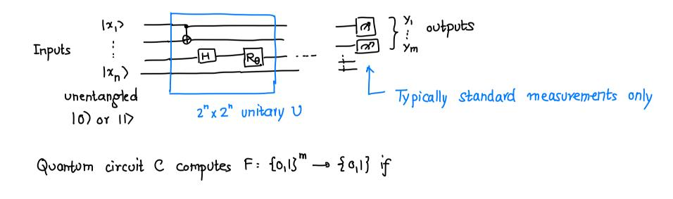
Typically we measure only at the end since we can add extra qubits to defer the measurement — "Principle of Deferred Measurement" Will be on HW 3
