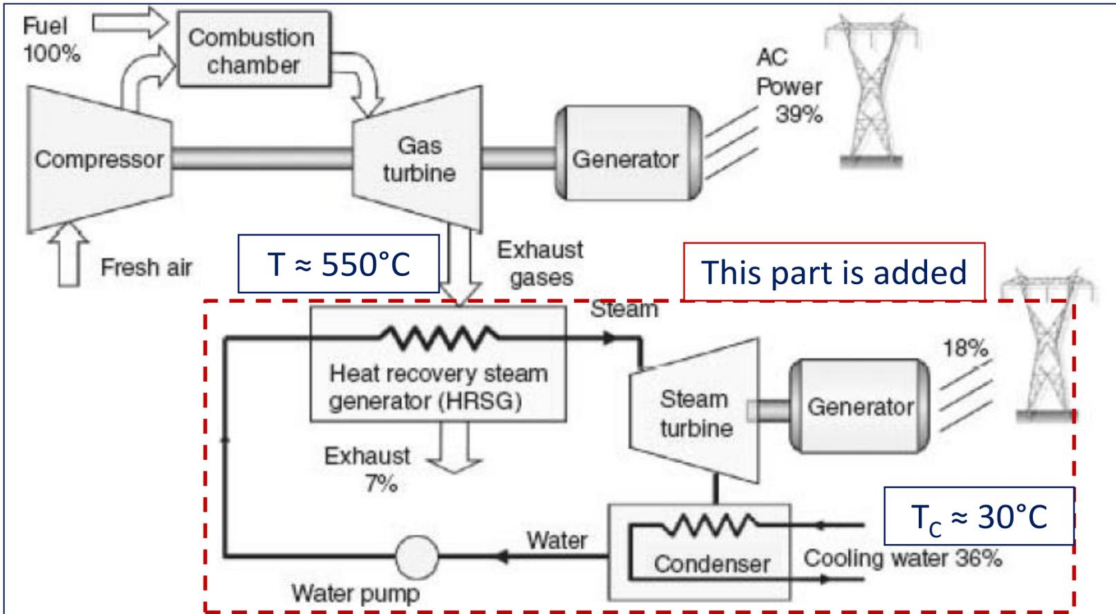
Efficiencies of up to 60% can be achieved, with even higher values when the steam is used for heating.
