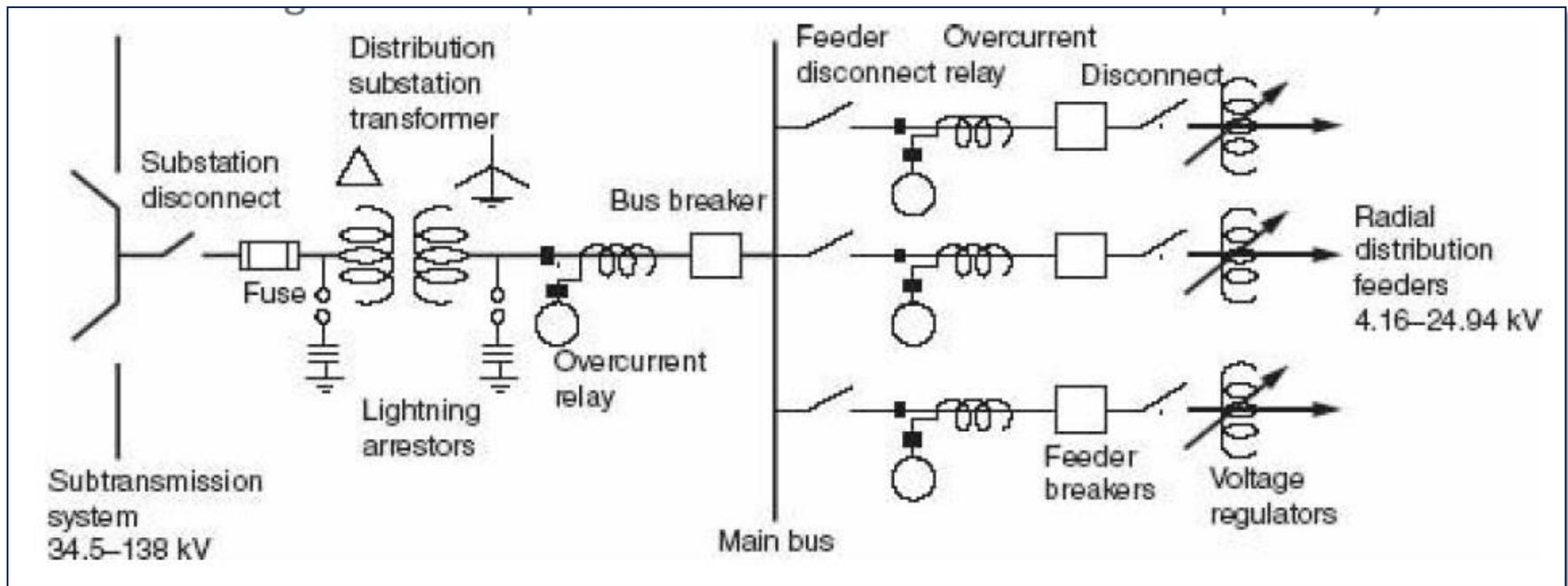
**FIGURE 1.5** A simple distribution station. For simplification, this is drawn as a *one-line diagram*, which means a single conductor on the diagram corresponds to the three lines in a three-phase system.
