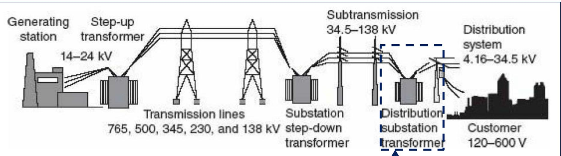
**FIGURE 1.6** Simplified power generation, transmission, and distribution system.
