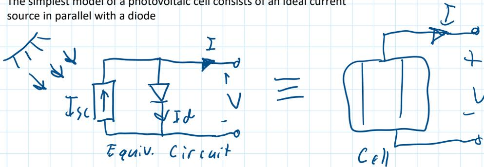
As with any other electric device, we want to obtain the V-I characteristics to compute currents, voltages and power once it is part of a larger circuit.
