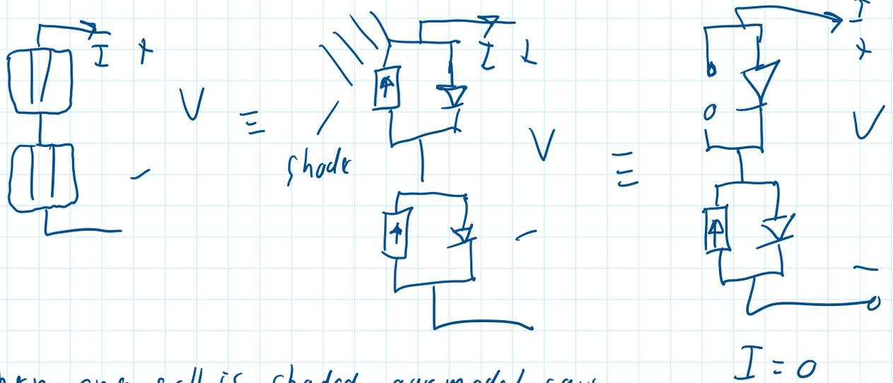
When one cell is shaded, our model says that  $I=0$ , while shading effects have a big impact on power output, it is not as dramatic as this simplified model suggests
