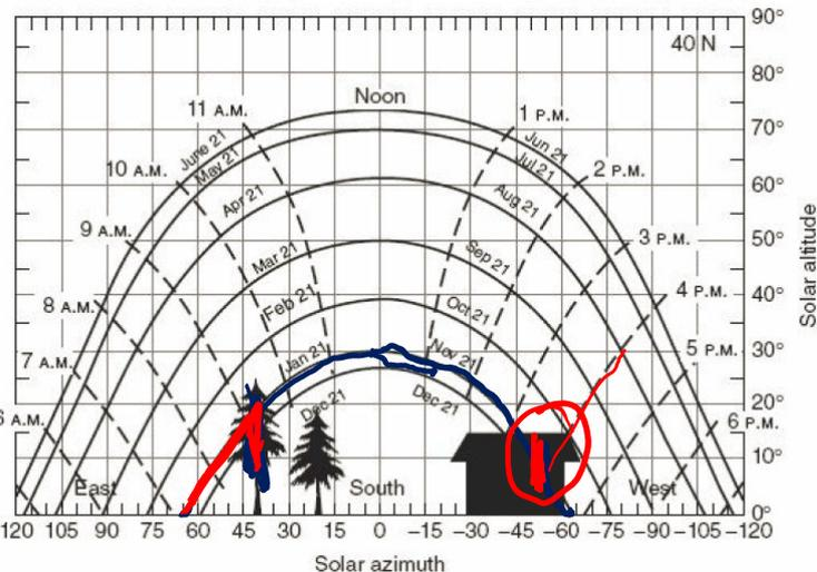
Ex. 4.4: January day; south-facing collector; at  $40^\circ$  N latitude with a fixed,  $30^\circ$  tilt angle.
