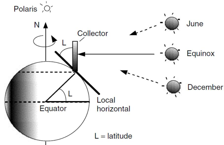
**Figure 4.8** A south-facing collector tipped up to an angle equal to its latitude is perpendicular to the sun's rays at solar noon during the equinoxes.
