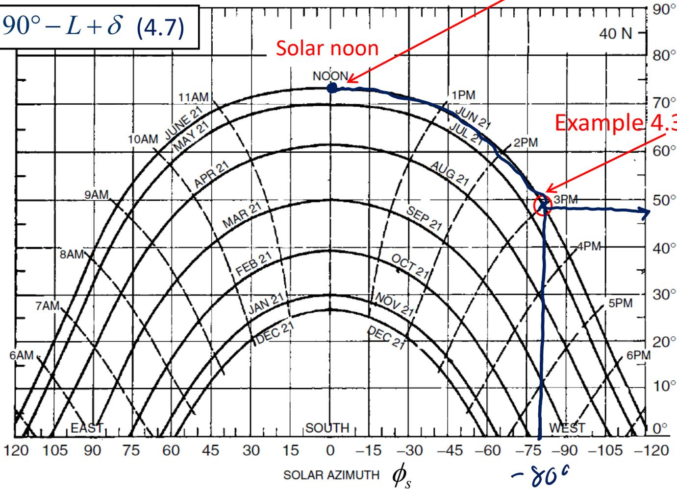
Figure 4.12 A sun path diagram showing solar altitude and azimuth angles for 40° latitude. Diagrams for other latitudes are in Appendix B.
