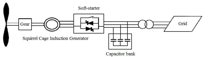
It is based on an induction generator connected with a fixed-speed wind turbine.
