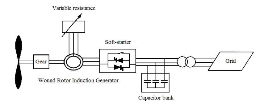
•The type B WECS (introduced by Vestas) generator is designed to work with limited variable speed wind turbine.
