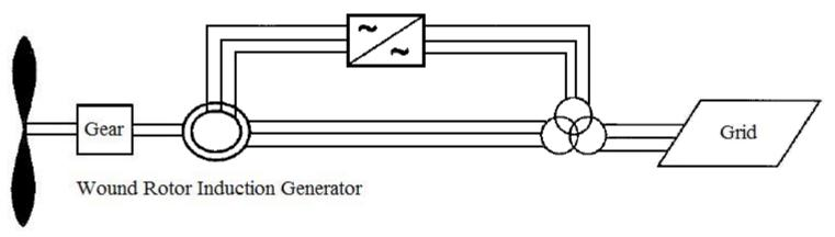
•This design uses two AC/DC converters with a capacitor between them to control the WECS. These converters are rated at 25% of total generator power.
