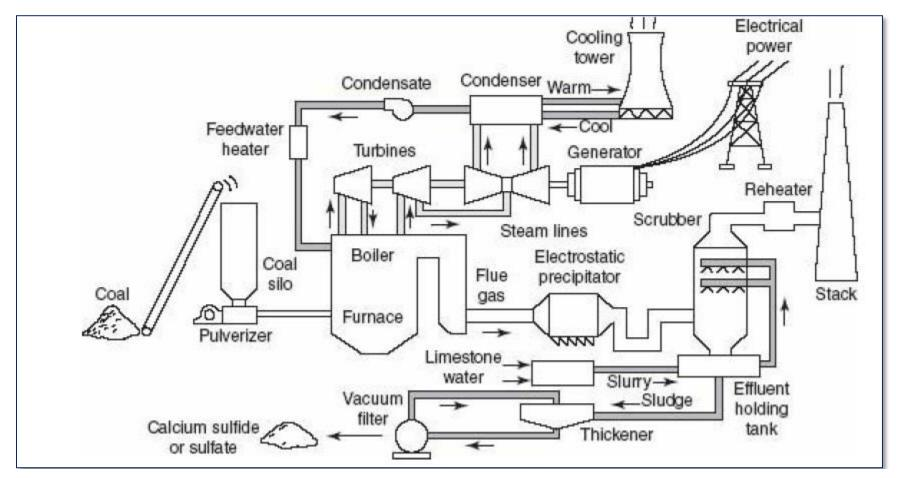
**FIGURE 1.21** Typical coal-fired power plant using an electrostatic precipitator for particulate control and a limestone-based SO<sub>2</sub> scrubber.
