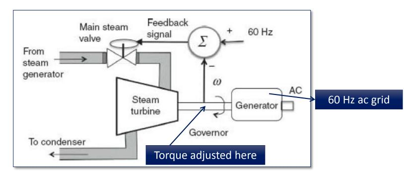
**FIGURE 1.9** Frequency is often automatically controlled with a governor that adjusts the torque from the turbine to the generator.
