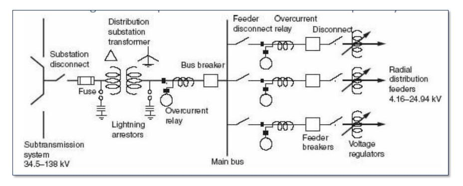
**FIGURE 1.5** A simple distribution station. For simplification, this is drawn as a *one-line diagram*, which means a single conductor on the diagram corresponds to the three lines in a three-phase system.
