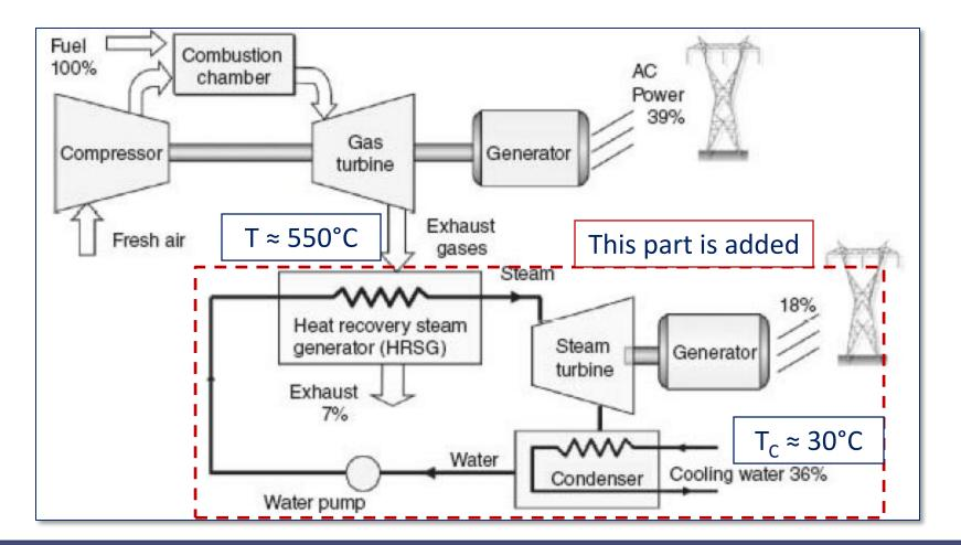
Efficiencies of up to 60% can be achieved, with even higher values when the steam is used for heating.
