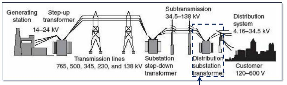
**<u>FIGURE 1.6</u>** Simplified power generation, transmission, and distribution system.
